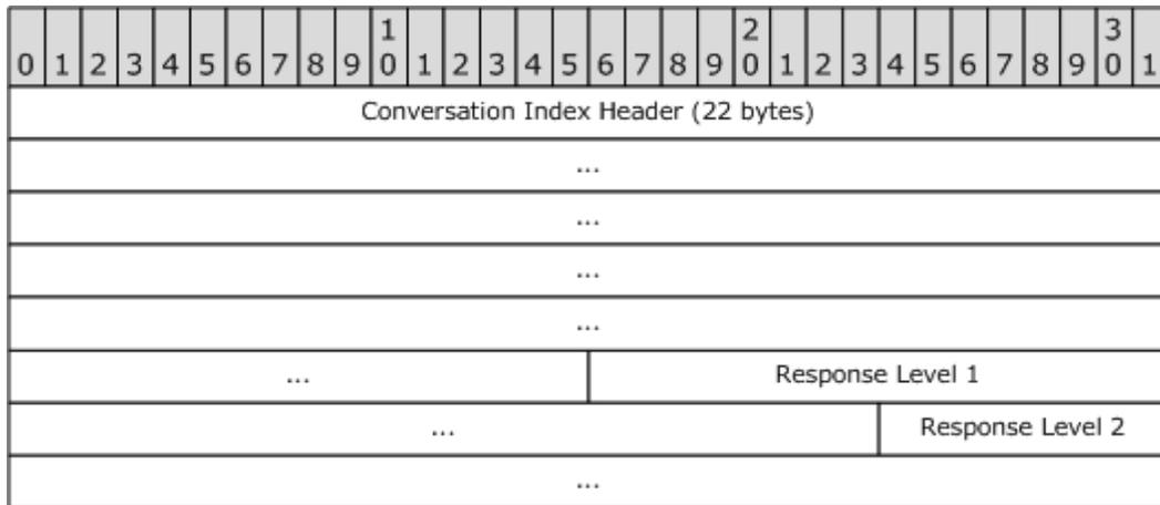
**Conversation Index Header (22 bytes):** Set according to the description in the following diagram.
