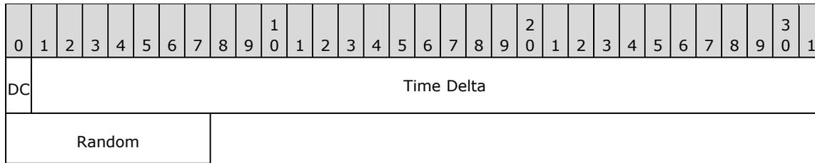
**DC (Delta code) (1 bit)** and **Time Delta (31 bits)**: Calculated based on **TimeDiff**, a 64-bit value representing the difference between the current time and the time stored in the conversation index header:
