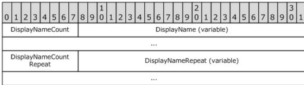
**DisplayNameCount (1 byte):** The COUNT ([MS-OXCDATA] section 2.11.1) of **Unicode** characters (not bytes) in the **DisplayName** field.
