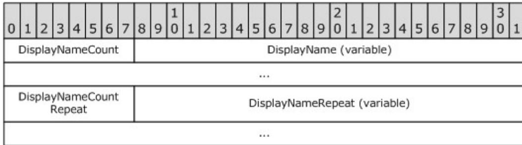
**DisplayNameCount (1 byte):** The COUNT ([MS-OXCDATA] section 2.11.1) of **Unicode** characters (not bytes) in the **DisplayName** field.
