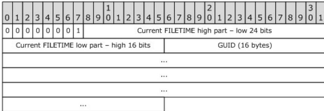
**Current FILETIME (40 bits):** The current time in **UTC** expressed as a **PtypTime** type ([\[MS-OXCDATA\]](#) section 2.11.1) is obtained, where only the 24 low bits of the high part and the 16 high bits of the low part of the **FILETIME** ([\[MS-DTYP\]](#)) are included in **Current FILETIME high part** and **Current FILETIME low part**, as shown in the following table.
