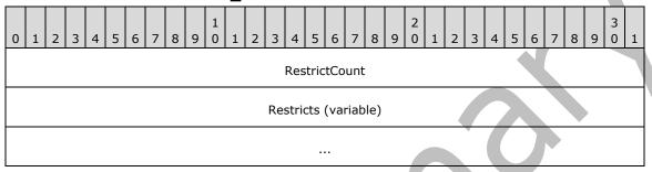
**RestrictCount (4 bytes):** Encodes the **RestrictCount** field of the **AndRestriction** structure, as specified in section 2.12.1.1. This value MUST NOT exceed 100,000.
