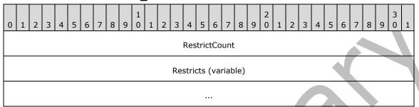
**RestrictCount (4 bytes):** This value encodes the **RestrictCount** field of the **OrRestriction** structure, as specified in section <u>2.12.2.1</u>. This value MUST NOT exceed 100,000.
