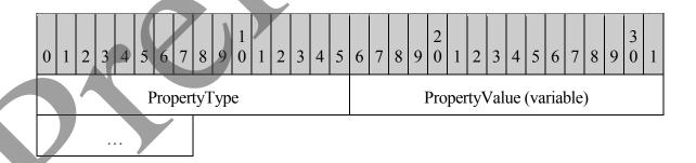
**PropertyType (2 bytes):** A 16-bit unsigned integer that specifies the data type of the property value, according to the table in section 2.13.1.
